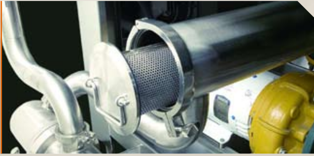
> Easy access stainless steel filter
